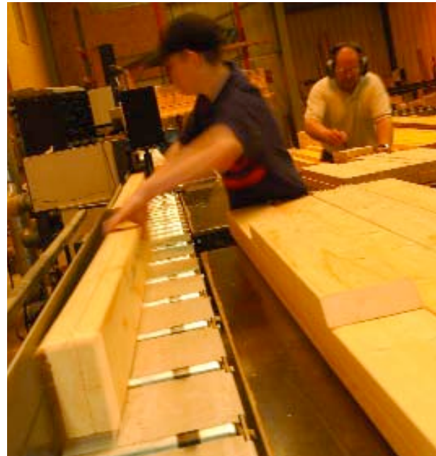
Cutting Crown FrameTherm to size to friction fit between narrowly spaced timber studs
