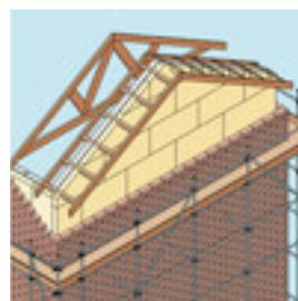
Figure 6. Installation of Batts in gable end wall
